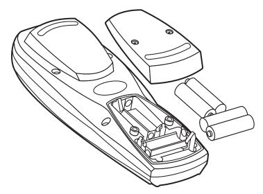
Figure 5. Battery Installation
