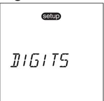
The digit selection allows the user to select the resolution of the reading, from 0.000, 0.00, 0.0 and 0 or auto resolution. Default is auto resolution.
