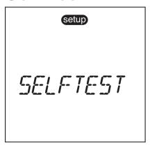
Puts the turbidimeter into a self-diagnostic mode. See the Turbidimeter Self Test section.
