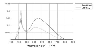
As can be seen from the graph, the white LED – Si photo detector system described here is quite broadband. Its appearance is very similar to that of a tungsten bulb and a cadmium sulfide photo detector combination. It also contains a narrow secondary peak at 460 nm. As the blue output is very limited in tungsten bulbs, this peak can aid in better detection of very small particles. However, as the peak area is very small compared to that of a main body, this enhancement is not very pronounced.
