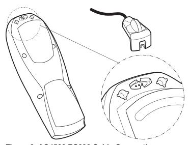
Figure 9. AQ4500 RS232 Cable Connection
