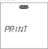
Allows the user to select the printout format. The user can select between a standard printout or a comma delimited format for importing data into a spreadsheet.
