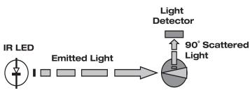
Figure 1. Pure Nephelometric Turbidity **Measurement without Color** Compensation
