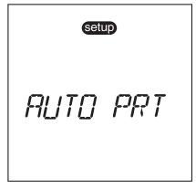
Auto print "ON" will automatically send readings to the printer.
