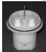
2. Press the diffusion tubing assembly onto the connector barbs, as shown in the figure below. The holes at the tubing ends press onto the barb fittings.
