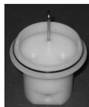
2. Insert the adaptors into the reagent bottle adaptor, as shown in the figure below, and hand tighten the adapters.
