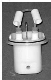
3. Press the diffusion tubing assembly caps onto the adaptors and loop the tubing onto the hook, as shown in the figure below.
