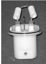
4. Press the diffusion tubing caps onto the adaptors and hook the tubing, as shown in the figure below.
