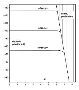
Figure 7 Precipitation of Cupric Ion by Hydroxide Ion
